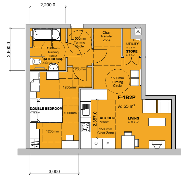
STANDARD 1BED ACCESSIBLE FLAT - POST CONVERSION
